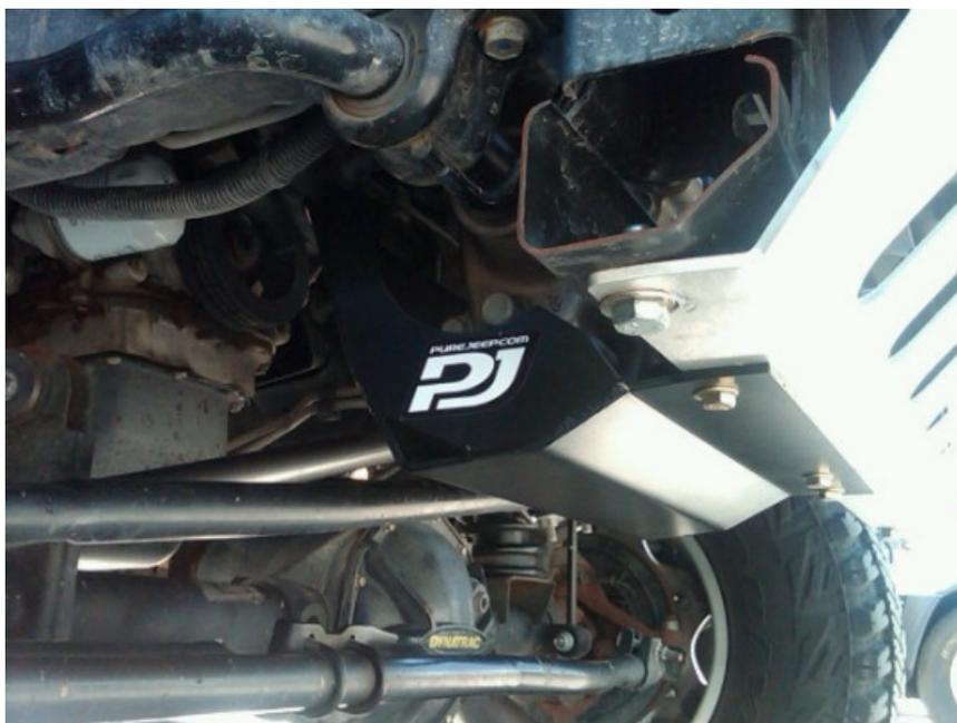
**Our skid for the electronic sway-bar found on the Rubicon JK models can be installed with (as shown) or without aftermarket front skid plates. Drilling is required in the stock under-rider support to properly mount. On some early model JKs, 1 of the necessary holes will be present. On most applications, all 3 holes will need to be drilled.**
